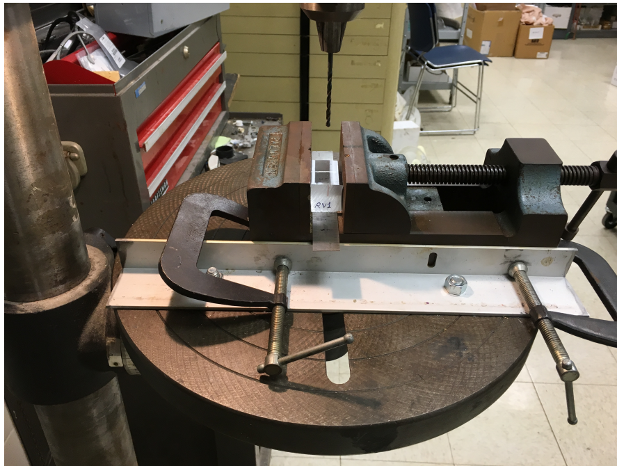
Figure 2. Positioning jig with acrylic block positioned for drilling.
